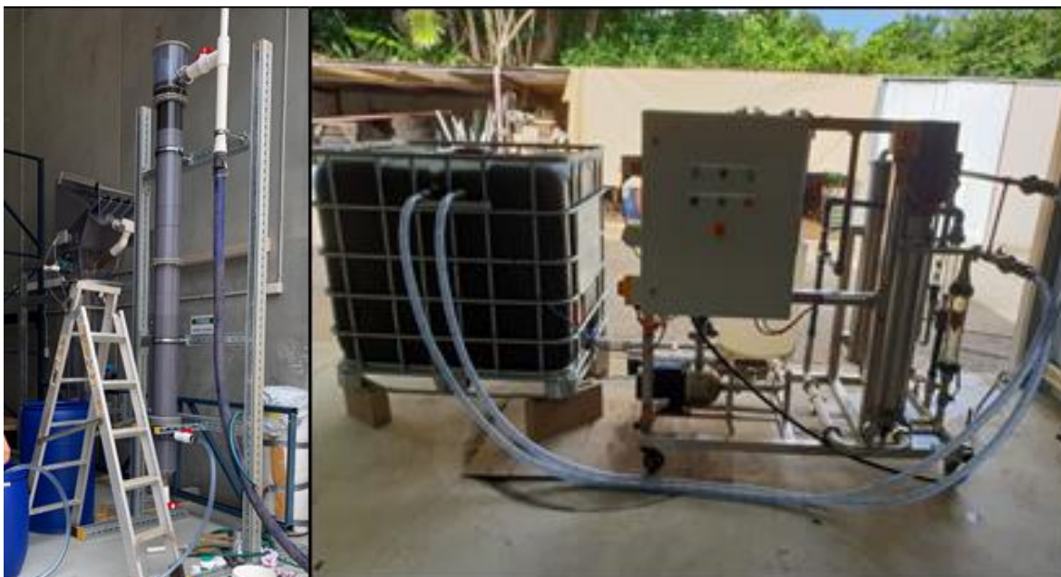
Figure 2. Photo of Site Piloting Equipment for Municipal Effluent Reuse, CIF (left), RO Unit (right)
