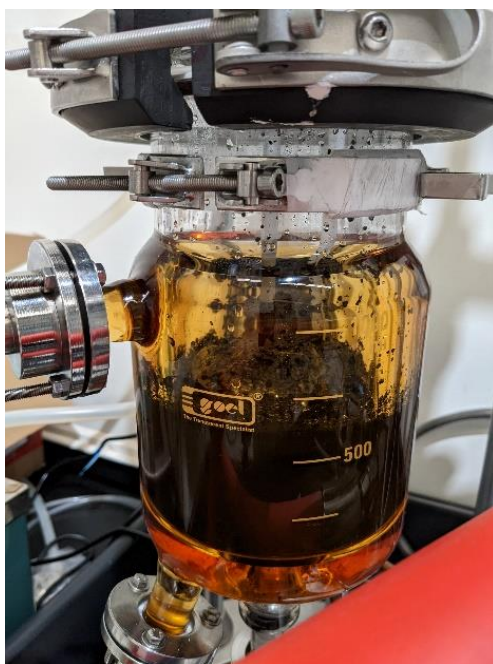
Figure 6: Black mass leaching – note frothing
