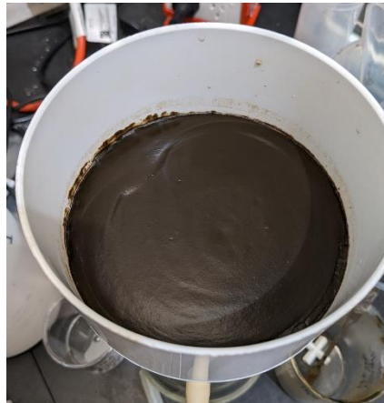
Figure 10: Bulk hydroxide precipitate from neutralisation of black mass PLS with NaOH
